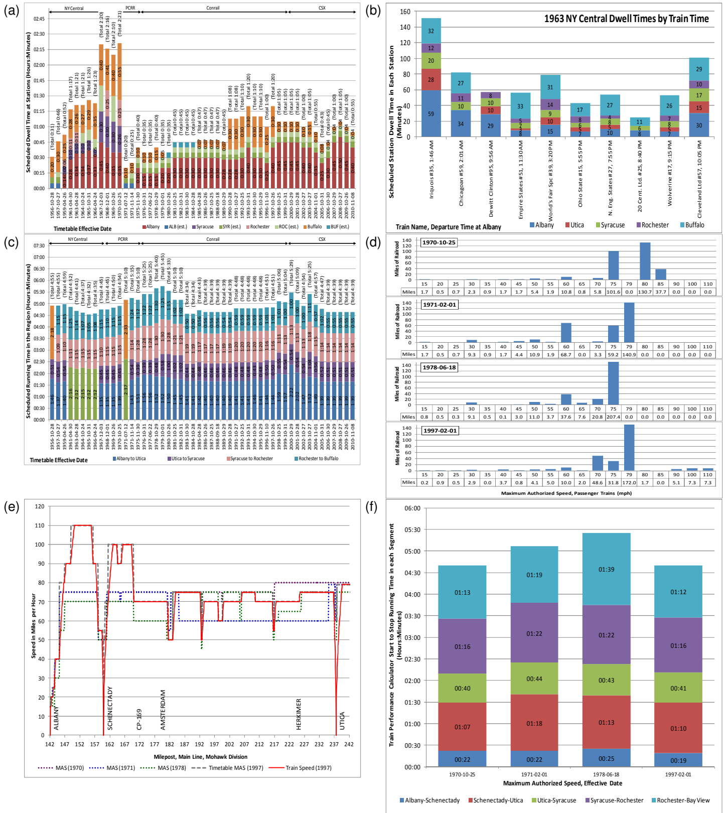
FIGURE 3 Longitudinal Analysis of Schedules and Speeds on the Penn Central Northeastern Region, Mohawk and Buffalo Divisions, 1956-2010: (a) Lake Shore Limited Dwell Time Analysis; (b) 1963 NY Central Railroad Dwell Time by Train; (c) Sectional Running Time Analysis; (d) Maximum Authorized Speeds; (e) Train Performance Curve from Albany to Utica; (f) Minimum Achievable Running Time per Simplified Train Performance Calculator.
