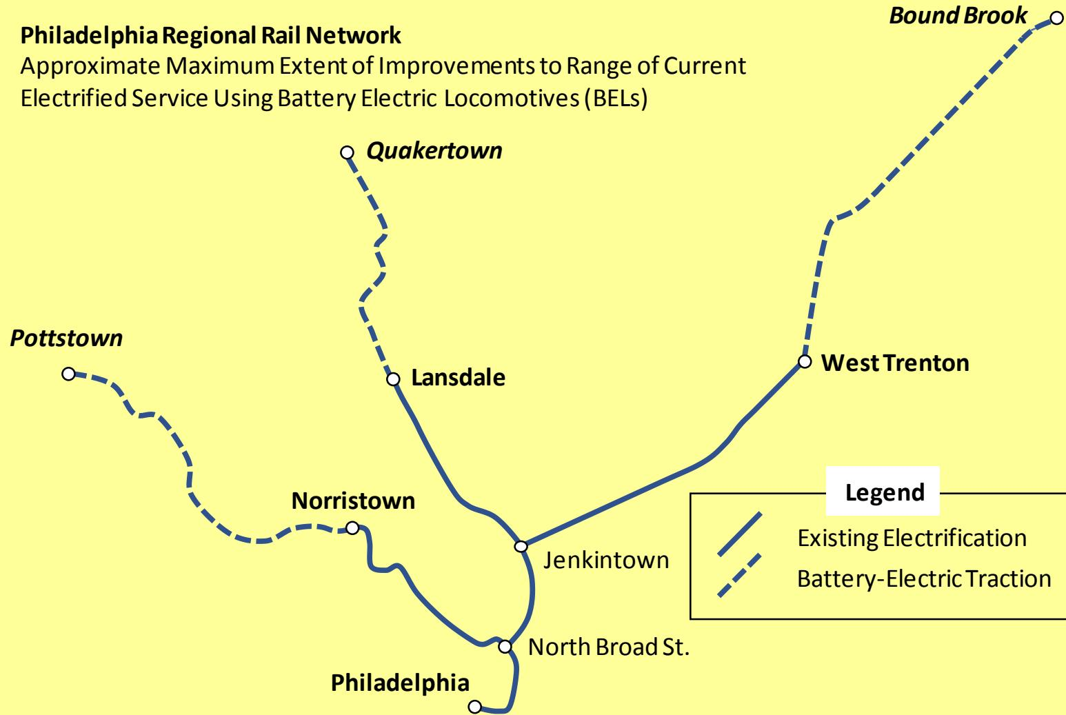
For Philadelphia, we examined another ability of battery-electrics: to extend the range of existing electrifications. We can operate off-wire on the former Reading side to Pottstown, Quakertown, and Bound Brook ...
