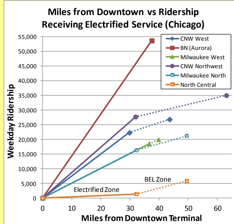
Even though we propose electrifying only about half the route-mileage, the vast bulk of the ridership will be in the electrified areas – the solid lines – versus the battery-powered zone with the dotted lines.
