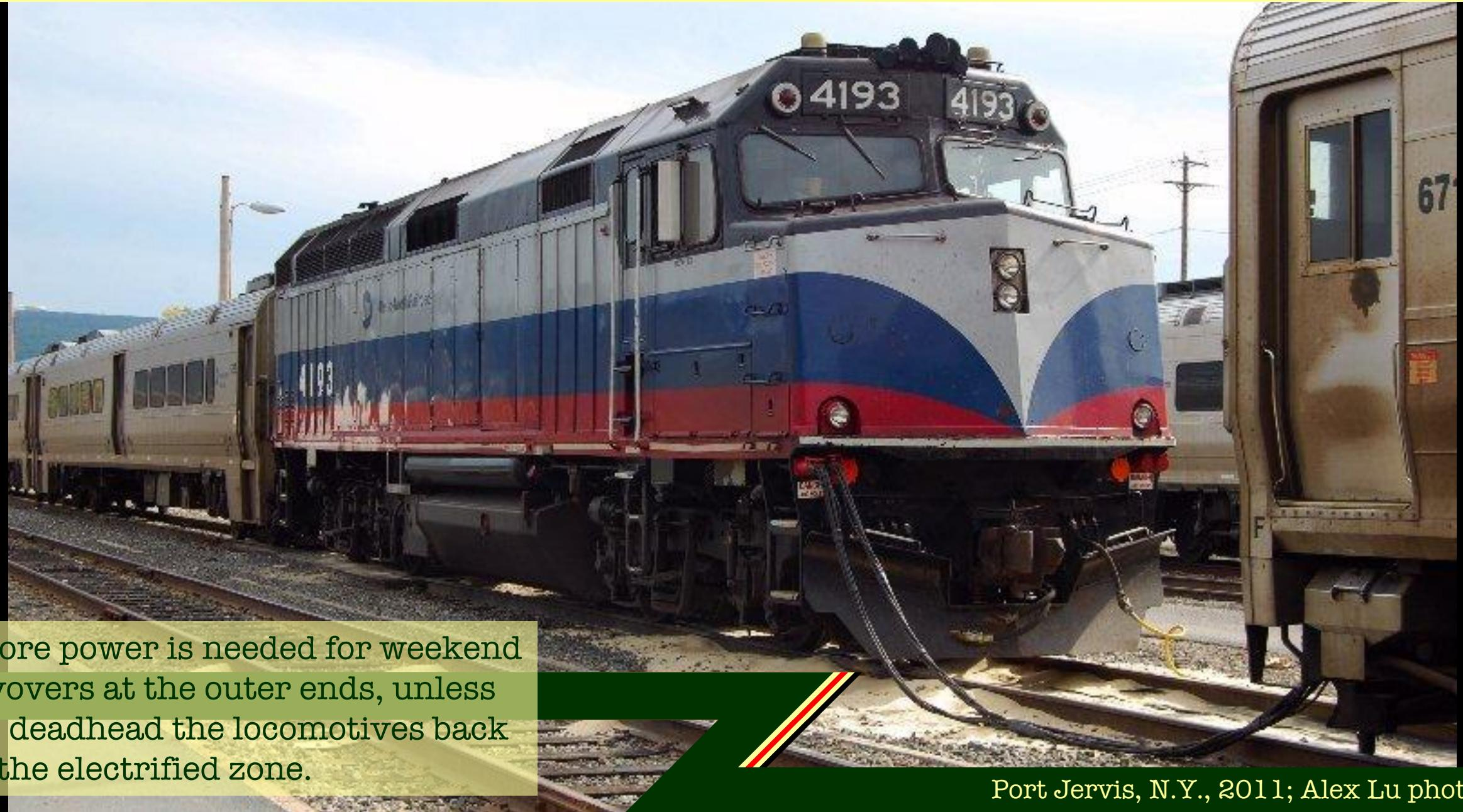
Shore power is needed for weekend layovers at the outer ends, unless we deadhead the locomotives back to the electrified zone.
