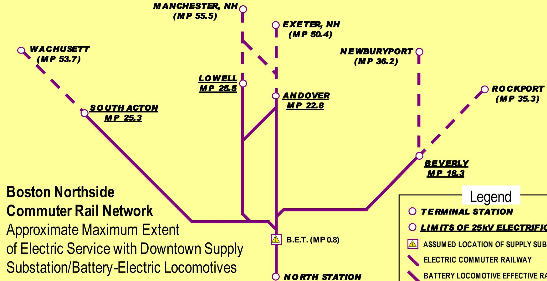
In Boston, we see what happens when a downtown supply substation pushes out 25 kV AC about 25 miles in any direction. This substation, in conjunction with autotransformer substations along the lines, can power electric service to South Acton and Lowell, as we see on the map. There is not quite enough range to reach Newburyport, Rockport or Haverhill, so we scaled back electrification to Beverly and Andover, with battery-electrics covering the remainder.
