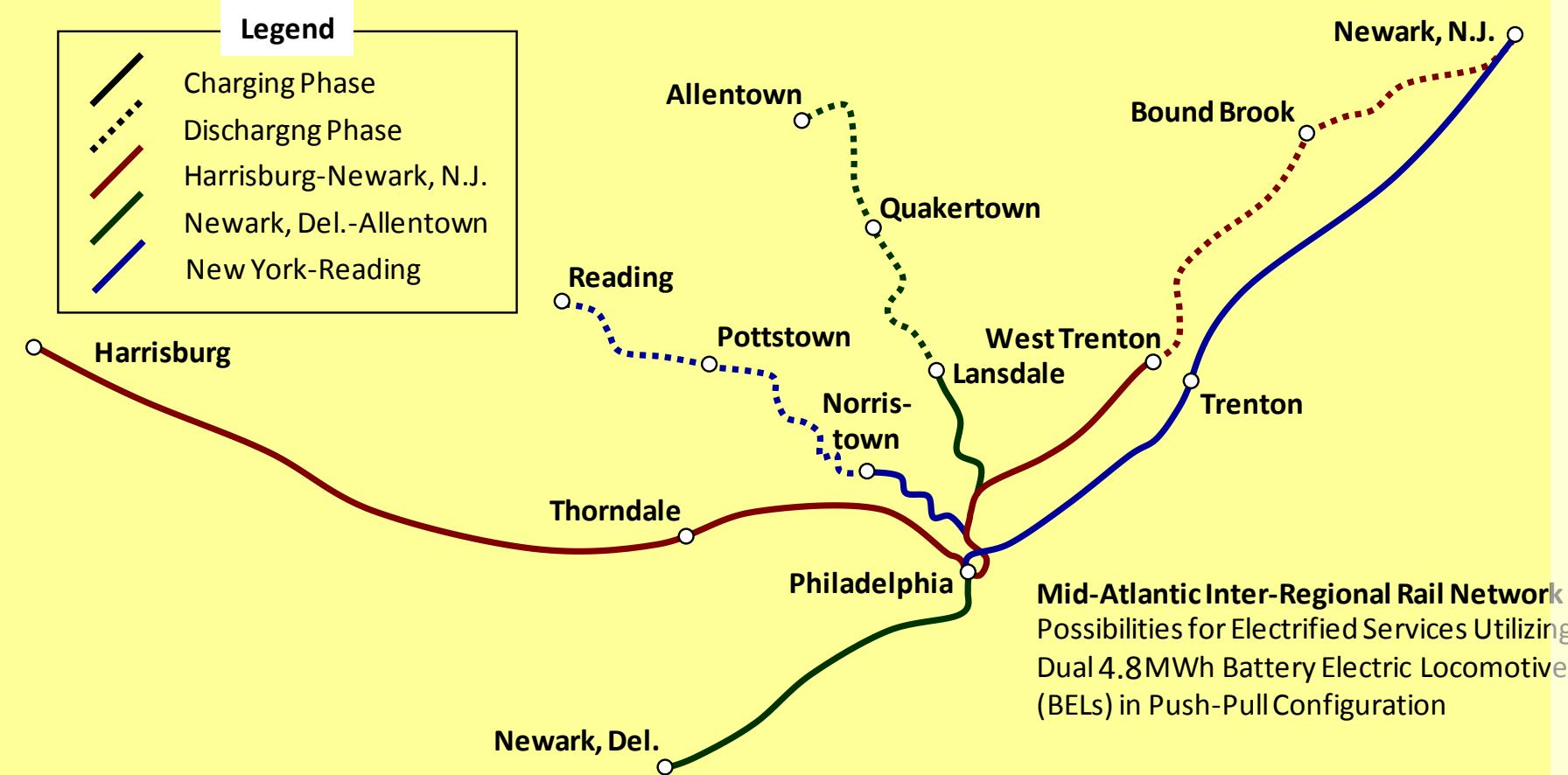
If trains spend enough time under the wire to recharge their batteries, we could take things even further, as with this proposed Mid-Atlantic Inter-Regional Rail system. Note that the line from Quakertown to Allentown has been abandoned and would need to be restored. Reading-side trains could reach the upper level at 30th Street Station via Market East and Suburban Stations, or go off-wire near Wayne Junction to reach Zoo Interlocking and the lower level at 30th Street.
