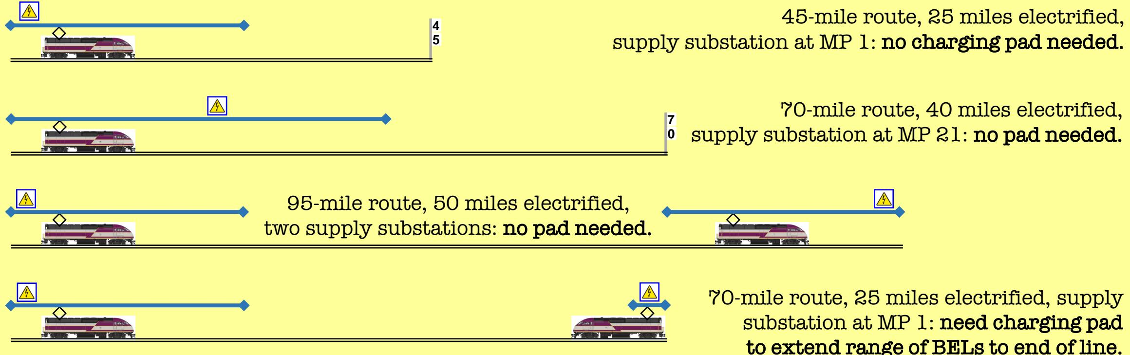
A charging pad is equivalent to a very short electrified segment tied to an additional substation.
