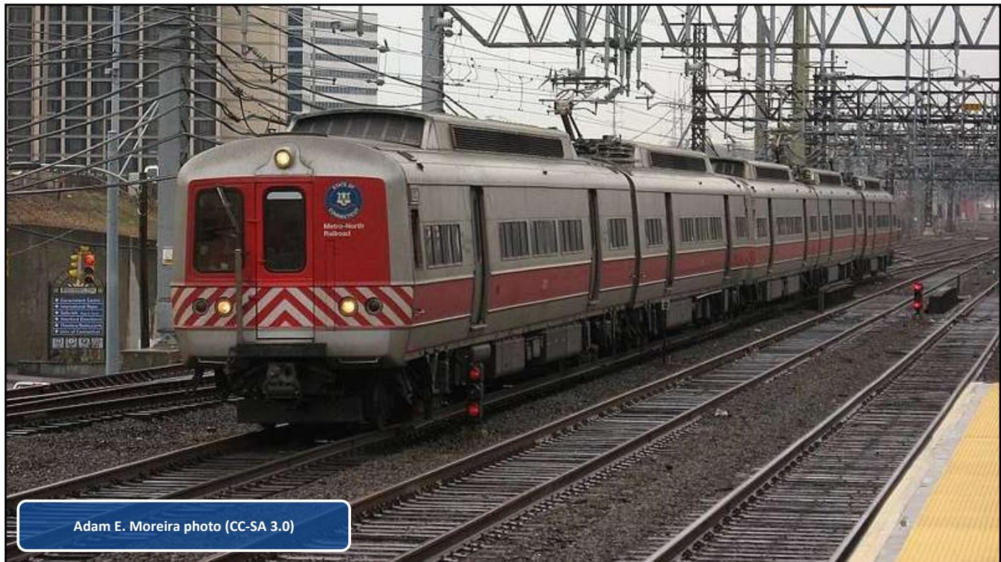
Some equipment have multiple pantographs bussed together. Allowing an electric train to travel across an air gap or section insulator between energized and de-energized sections momentarily allows two sections to be electrically connected, resulting in backfeeding through the high voltage bus onboard the train.
